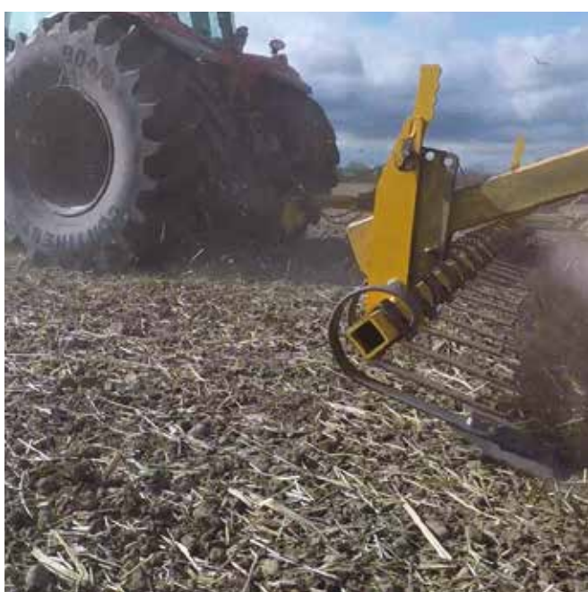
The Pro-Til's seeding arm ensures accurate depth and excellent seed-to-soil contact.
