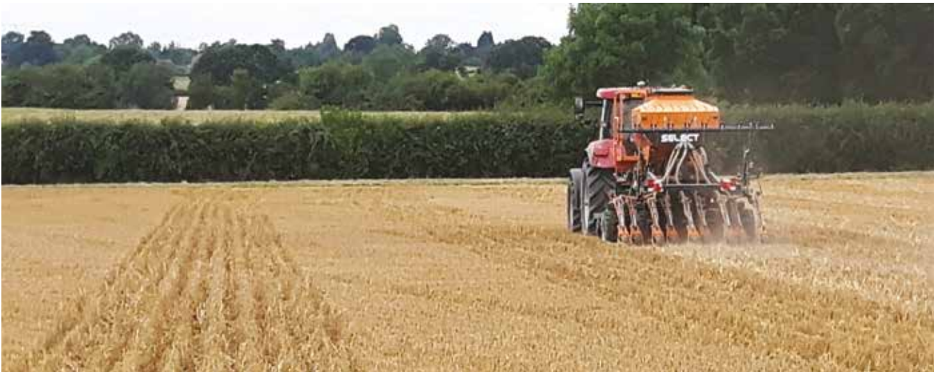
The new low disturbance coulters on the Pro-Til 3T Select working a dream
