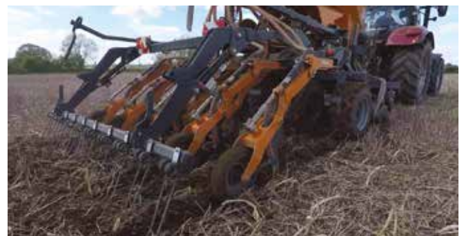
The Pro-Til's seeding arm ensures accurate depth and excellent seed-to-soil contact.
