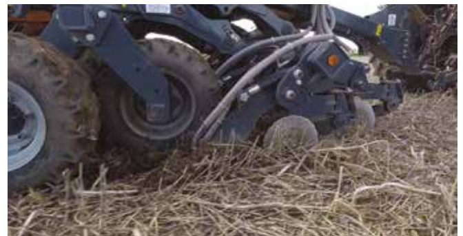
Front discs and leading tines prepare the perfect seeding strip, complete with a dose of fertiliser for a quick root boost.
