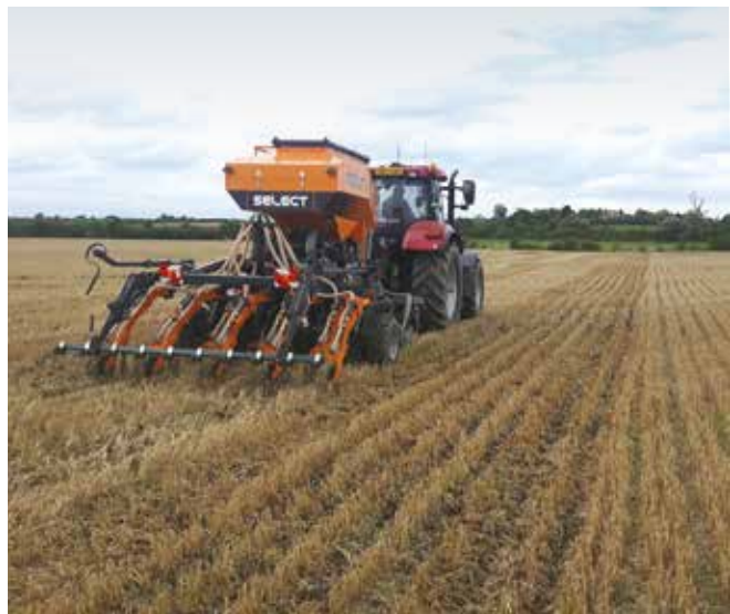
Pro-Til Select is now capable of direct drilling, as well as strip tilling.
